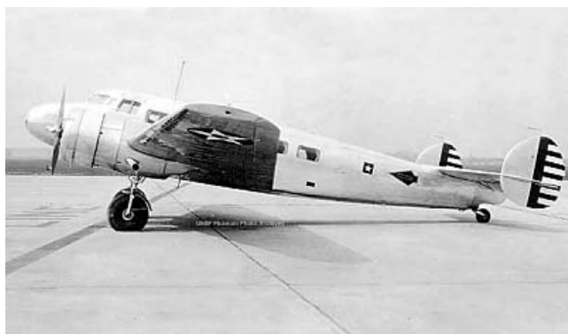
The military version of the L-10A: Y1C-36 of the US Army Air Corps (UAAC)
